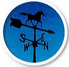
Wind direction can be observed with a weather vane. The arrow points toward the direction the wind comes from. That is, it points into the wind. The vane below shows that there is a northerly wind. The name of the wind is the direction from which it blows. A north wind comes from the north and moves toward the south.
